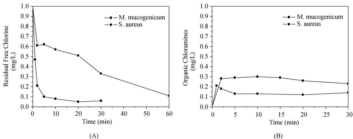
**Figure 4.** (A) Free chlorine decreased with time during the inactivation experiments of *S. aureus* and *M. mucogenicum*. (B) Formation of organic chloramines during the inactivation process of *S. aureus* and *M. mucogenicum*. Note. Initial concentration of *M. mucogenicum* and *S. aureus* were  $1.2 \times 10^7$  CFU/mL and  $1.4 \times 10^7$  CFU/mL respectively.
