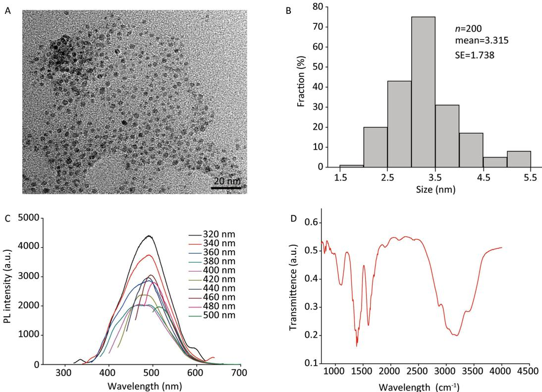
**Figure 1.** Characterization of graphene quantum dots (GQDs). (A) TEM image of GQDs (scale bar=20 nm); (B) Size distribution of GQDs; (C) PL intensity of GQDs; (D) FTIR spectra of GQDs. TEM, transmission electron microscopy; PL, photoluminescence; FTIR, Fourier transform infrared.
