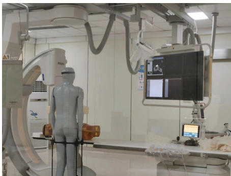
Figure 1. Experimental setup involving two anthropomorphic phantoms for measuring scattered radiation doses during interventional procedures.
