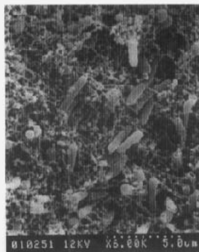
FIG. 4. Immobilized microbial cells inside the PVA gel.
