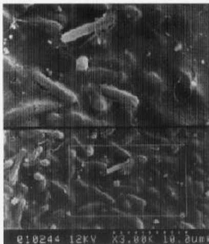
FIG. 3. Immobilized microbial cells on the surface of PVA gel.
