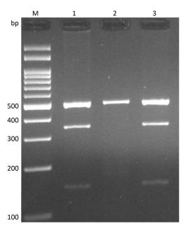
**Figure 2.** Detection of the *TLR1* rs5743618 polymorphism by electrophoresis of the polymerase chain reaction-restriction fragments length polymorphism assay products. The G allele is digested by Pstl restriction enzyme into 351- and 149-bp products, whereas the T allele remains undigested (500 bp). M: DNA marker; lanes 1 and 3: TG; lane 2: TT.
