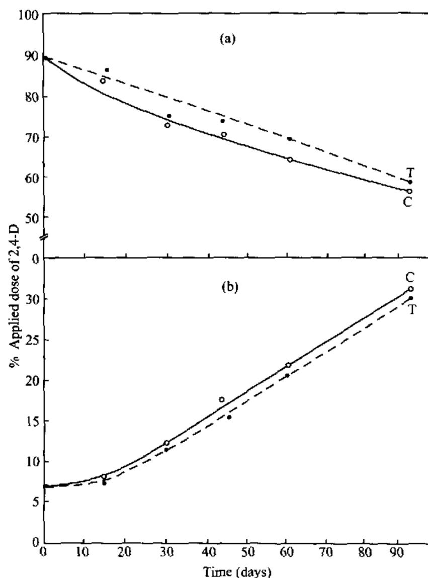
FIG.2. <sup>14</sup>C-Methanol extractable (a) and <sup>14</sup>C-bound residues (b) in Clay loam soil spiked with <sup>14</sup>C-2,4-D under anaerobic Conditions during 12 weeks. C=Control, T=Treated.
