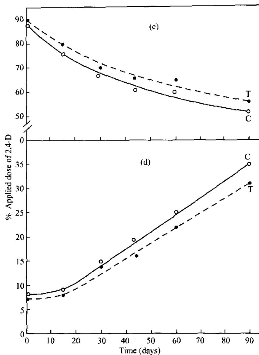
FIG.3.  $^{14}\text{C}$ -Methanol extractable (c) and  $^{14}\text{C}$ -bound residues (d) in Clay soil spiked with  $^{14}\text{C}$ -2,4-D under anaerobic Conditions during 12 weeks. C=Control, T=Treated.
