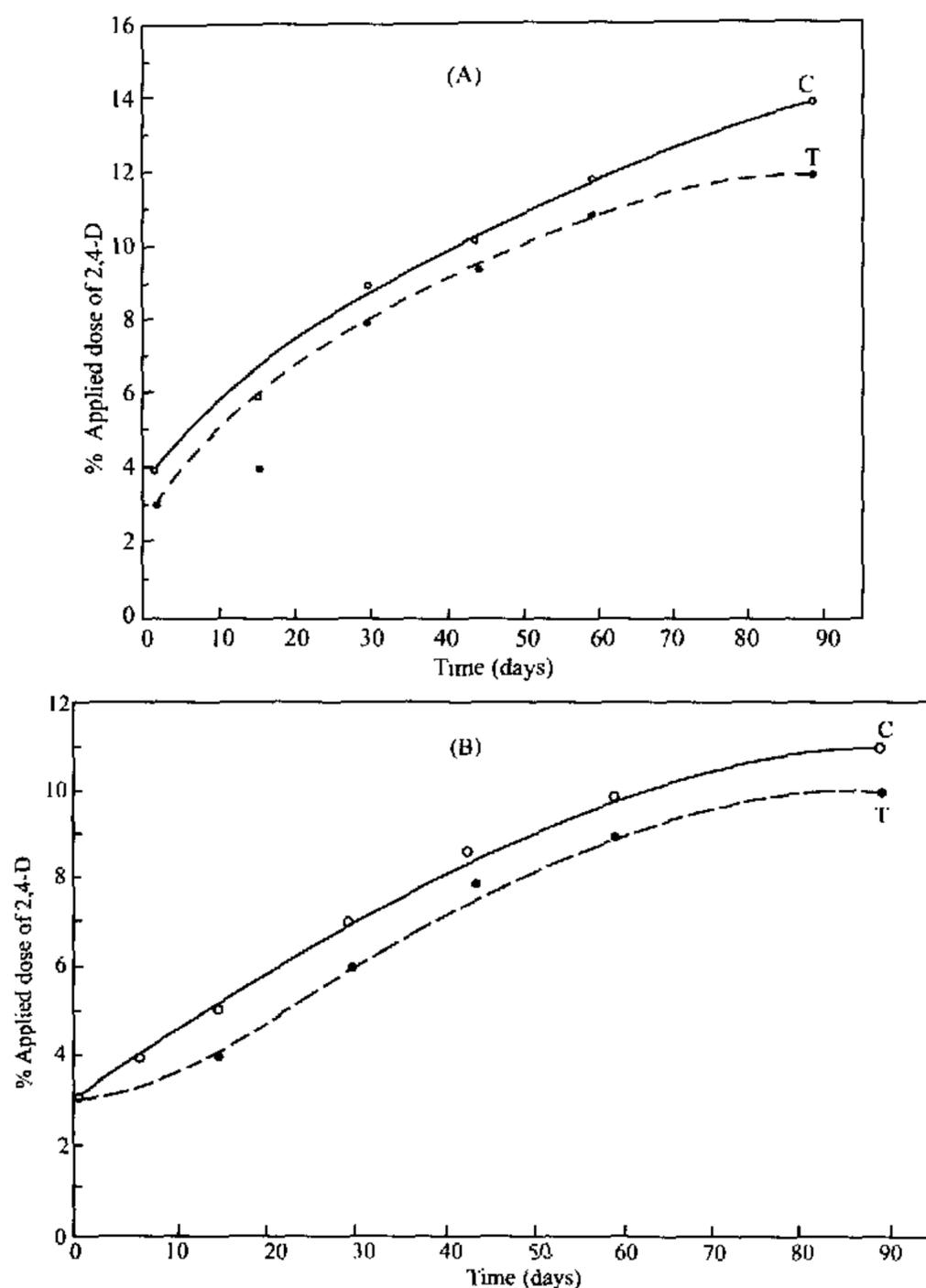
FIG.1. Cumulative  $^{14}\text{CO}_2$  for clay (A) and clay loam (B) soils spiked with  $^{14}\text{C}$ -2,4-D under anaerobic conditions during 12 weeks. C=Control, T=Treated.
