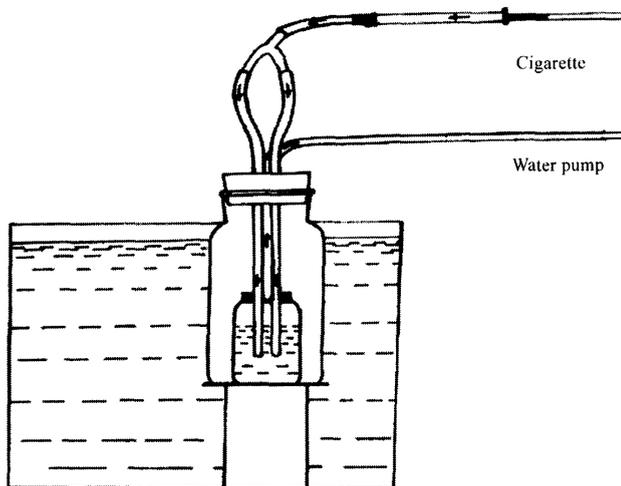
FIG.1. Apparatus used for the preparation of CSE solutions. Cigarette smoke was bubbled through the buffer (10 mmol/L HEPES, pH 7.4) at one cigarette per 5 minutes using a simple three-way pipe with a cigarette inserted into a holder attached to one pipe and the other two pipes going to a 60 mL brown glass bottle with 30 mL buffer in a water bath at  $37^\circ\text{C}$ , and the left pipe was driven by a water pump (constant pressure at  $-5\text{ cm H}_2\text{O}$ ).
