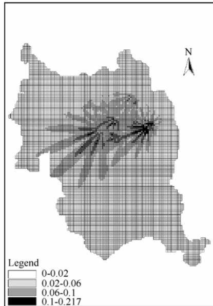
FIG. 1. The sulfur dioxide pollute concentration fields of studied region of simulation (mg/m<sup>3</sup>).
