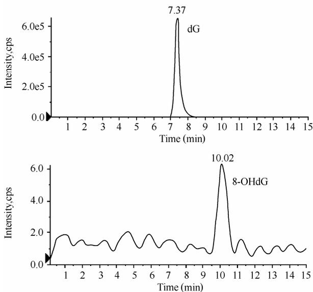
FIG. 5. Representative HPLC-MS/MS chromatogram for a control in MRM mode (The transitions monitored for 8-OHdG and dG see Fig. 4).
