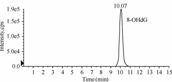
FIG. 4. Chromatogram of the standard solution of 8-OHdG (150 mg/L) and dG (50 mg/L) in the MRM mode using HPLC-MS/MS. Under the HPLC conditions used, 8-OHdG and dG were eluted at 10.02 and 7.37 min, respectively. 8-OHdG and dG were monitored by four pairs of transitions (284.3/168.4, 284.3/140.2, 306.1/190.2, and 306.1/262.1) and three pairs of transitions (268.5/152.2, 268.5/135.3, and 268.5/117.3), respectively.
