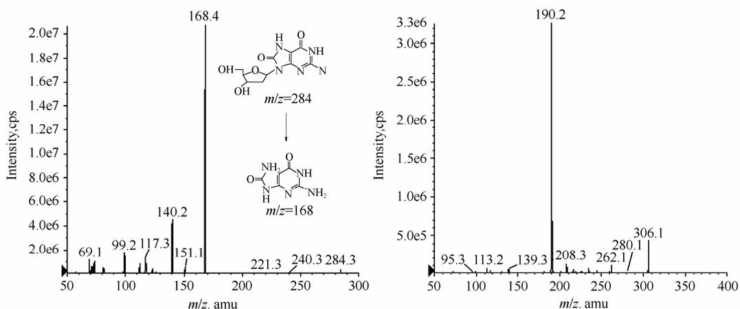
FIG. 2. Positive electrospray ionization mass spectrum (MS/MS) of 8-OHdG. A: product ion scan of  $[M+H]^+$  ( $m/z$  284.3); B: product ion scan of  $[M+Na]^+$  ( $m/z$  306.1).
