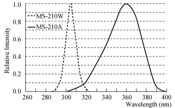
**Figure 1.** Spectral sensitivity of UV radiometers (MS-210W and MS-210A).
