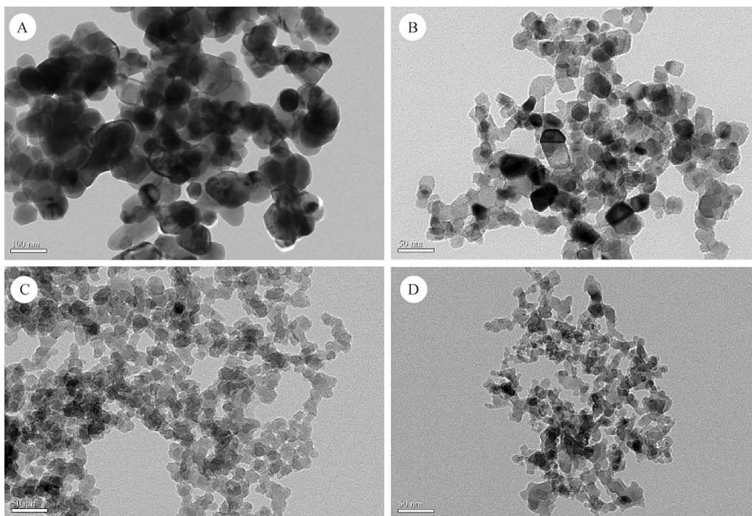
**Figure 1.** TEM analysis of nanomaterials. (A) ZnO, (B) TiO<sub>2</sub>, (C) SiO<sub>2</sub>, and (D) Al<sub>2</sub>O<sub>3</sub>. Original magnification  $\times 120\,000$ .
