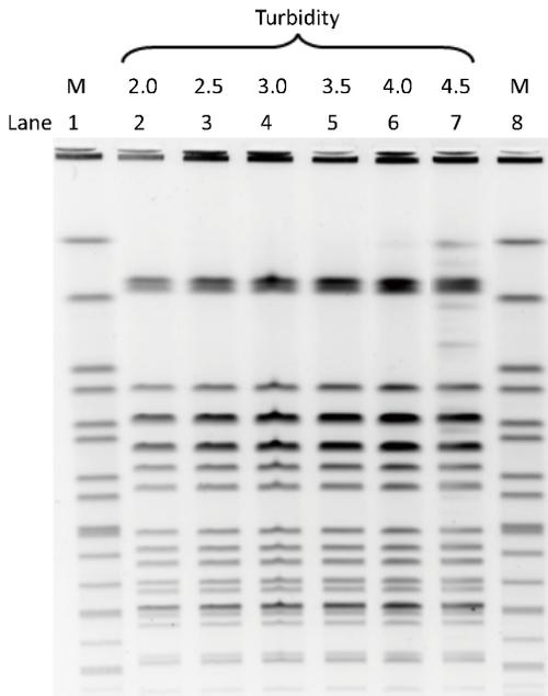
**Figure 2.** PFGE gels showing a comparison of plugs made with different cell suspension concentrations (Lanes 2-7, strain CF72, *Xba*I digestion). The size standard (*Salmonella enterica* serotype Braenderup strain H9812, *Xba*I digestion) was loaded in Lanes 1 and 8. The electrophoretic parameter was 6.8 s-34.8 s for 19 h.
